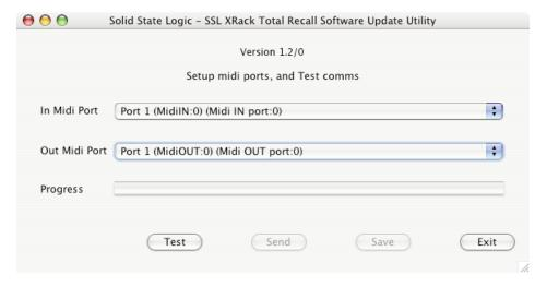
5. Go to the In MIDI Port menu. Select the MIDI IN port which is connected to your X-Rack from the drop down list. In the example shown below this was 'port 1' on an 8-Port interface. If nothing appears in the list check that you have installed the files listed in the **System Requirements** section opposite.
