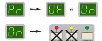
When set to '@r' the Save and Delete functions are disabled. When set to '@F' they are enabled. The 'Wr Prot' LED lights to show this mode has been selected.
